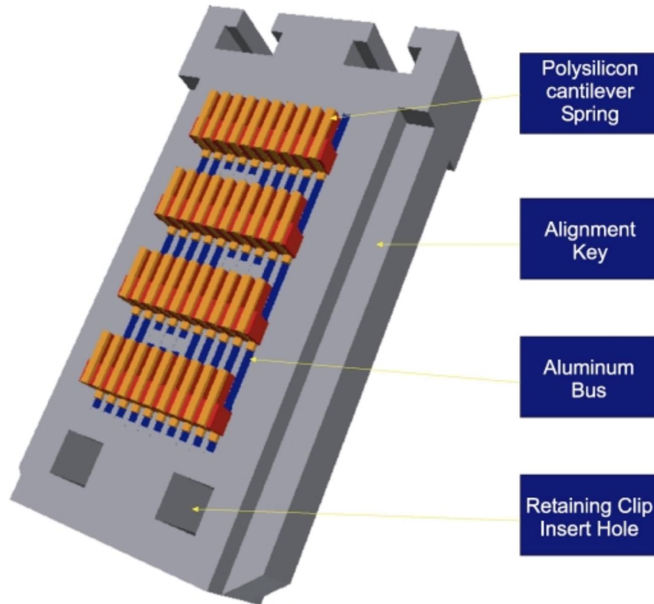
Microbus Card 3-D model Before Heat Treatment. Generated by IntelliSuite Design Tools Simulating Fabrication Processes
