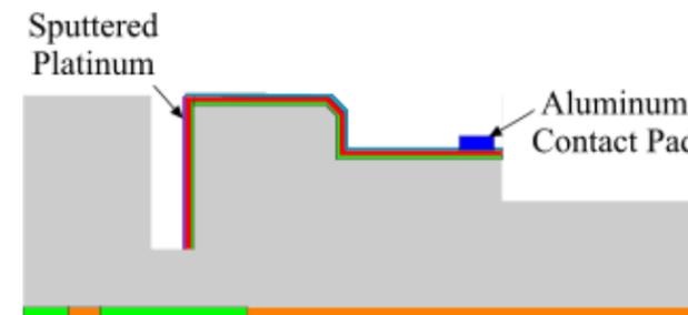
75x75 μm<sup>2</sup> Aluminum contact pads are then formed. 200 nm thick platinum is then sputter deposited in the interconnection shaft and patterned using an electrodeposited photoresist.
