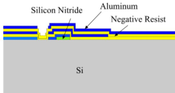
70 nm thick PECVD silicon nitride is deposited, patterned and etched on the top of a 400 μm thick silicon wafer. Three layers of aluminum-negative photoresist laminations are deposited.
