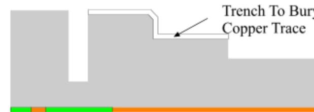
PECVD nitride on the wafer topside is removed. The wafer is TMAH etched to form the slant corner on the top. The wafer is then RIE etched to form 5 μm deep by 35 μm wide trenches.
