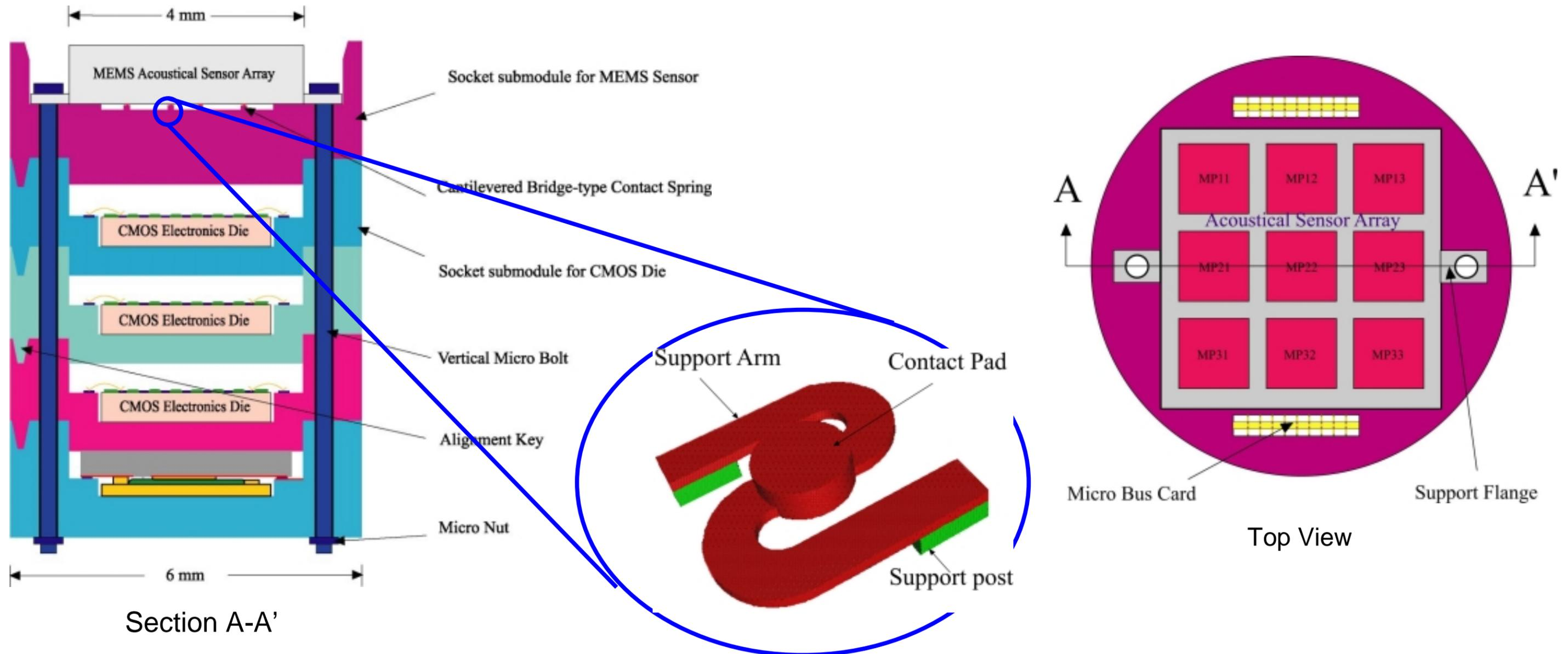
The MEMS Sensor is surface mounted to a socket submodule
