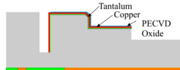
Tantalum is sputter deposited and patterned in the trenches. 1.0 μm thick copper is sputtered and patterned. Finally a 3.5 μm thick silicon dioxide is PECVD deposited to protect the copper traces from oxidation.
