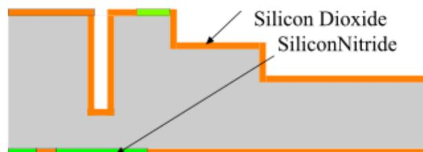
70 nm thick PECVD nitride is then deposited and patterned on the wafer backside. Thermal oxide is grown on both sides of the wafer and patterned.
