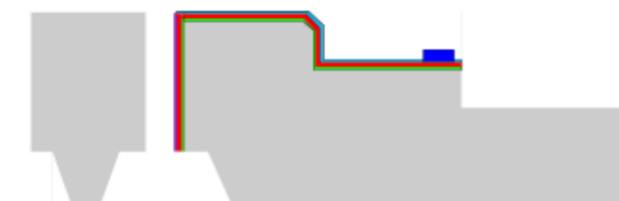
Wafer backside nitride is stripped. Anisotropic etching is performed on the wafer backside using TMAH to complete the fabrication process.
