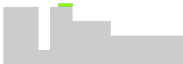
After the 3rd ICP-RIE process, the wafer patterning is completed. The 3rd Aluminum mask is then stripped.
