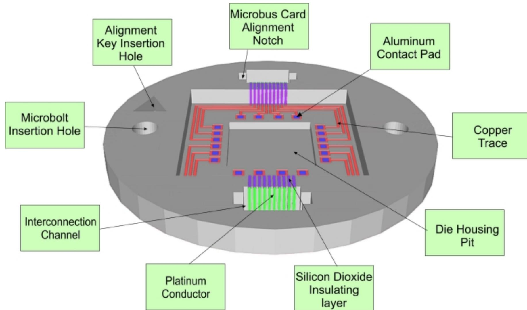
3-D model of a die container type MEMS socket submodule after simulating the fabrication processes using IntelliSuite design tools
