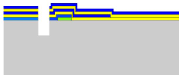
O<sub>2</sub> ashing of the negative photoresist is carried out by ICP-RIE method. The wafer is then successively ICP-RIE etched using Aluminum and negative resist laminations as delayed mask.
