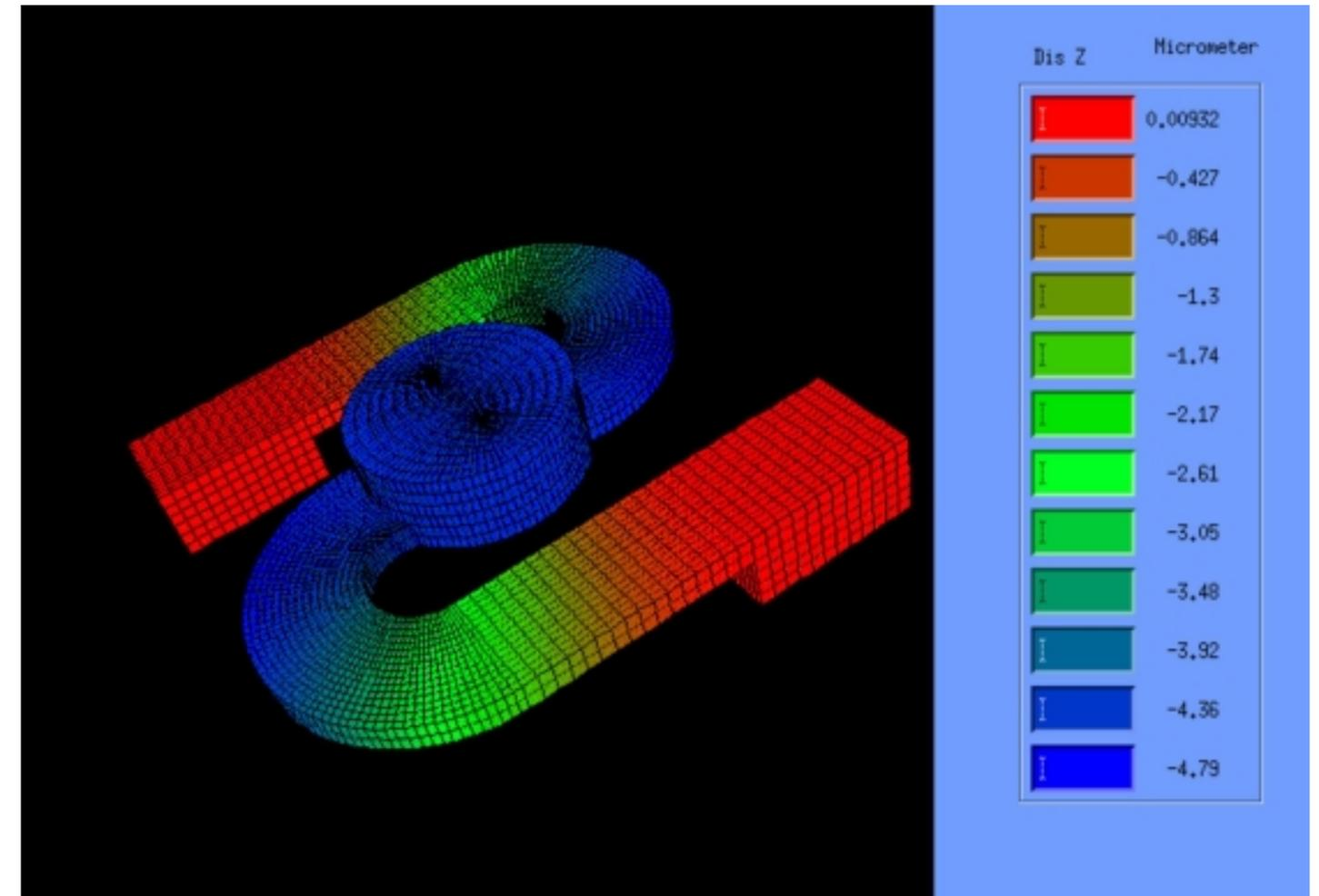
Z-axis displacement is uniform throughout the contact pad area
